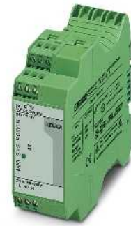
Power supply unit, 1 AC, 24 V DC, 1.5 A, flat design, optional DIN rail connector
